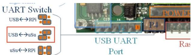
Step 2: Connect Edu board with a USB to serial port cable. Check the device id, and change the following line in flashWriter.py to the right one:
